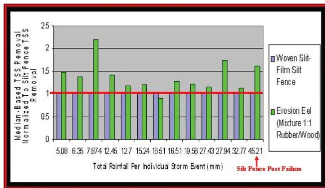
Field testing demonstrates the EELs consistently outperform silt fence during real storm events.
