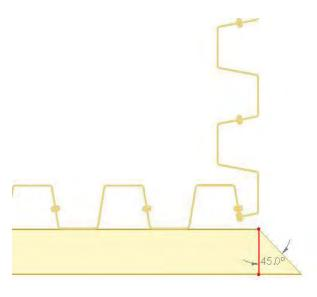
You might want to go ahead and cut your other mitered corner piece as well, since you are already cutting. You should have enough material to cut from a new section so that your face joints are as far from the corner as possible. For this cut you will make the matching miter cut 22.5 or 45 degrees from perpendicular, respectively, for a 45 or 90 degree turn.
