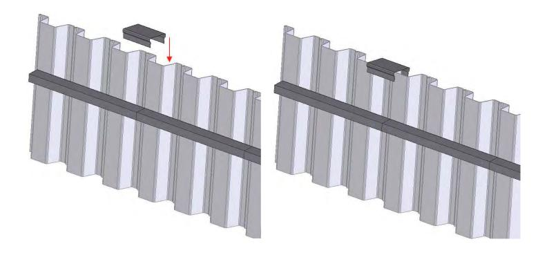
Next, slide a ShoreGuard Cap section onto the insert. The cap acts like a roof on your wall, so you want to make sure that no wall is left exposed underneath the outside end of your cap.
