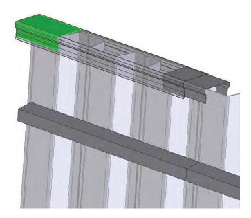
After you have secured the cap to the wall in a level position, you will need to remove the temporary leveling insert as you will be installing it at a later time.
