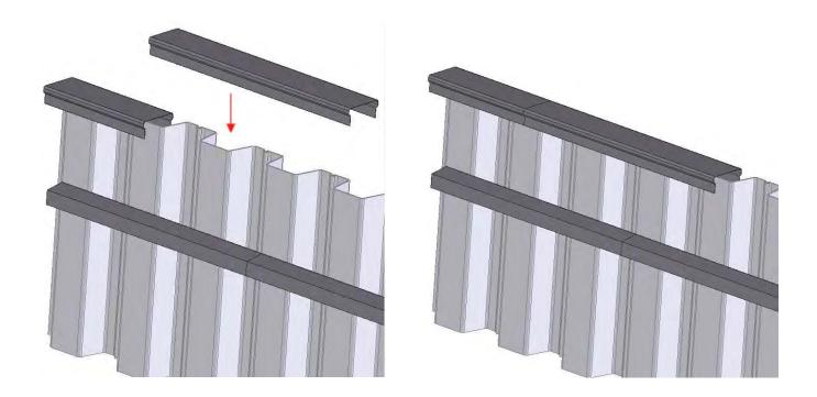
Slide a 20' cap section onto the cap inserts. Because your cap system acts like a roof, be sure that the outside end of your wall is completely covered by the cap section. Because you have made this 10' insert piece, every other insert will automatically be half-in, half-out of the cap for optimal placement.
