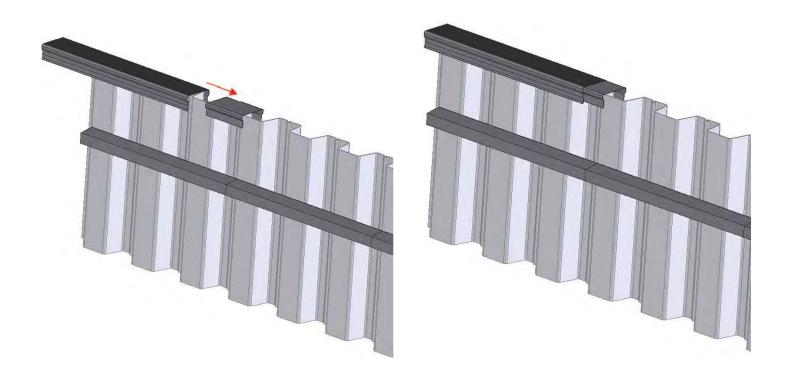
The cap is designed to be wider than the sheet piling wall that it houses. This allows for easy installation and overhanging material for increased protection. Throughout this entire capping process, you will probably want your cap's contact with the sheet piling to be on the front face (exposed side). This is a must if you are planning on tying back through the cap, and this is the way it will be shown throughout the manual. There will also be some instances were there is no gap between
