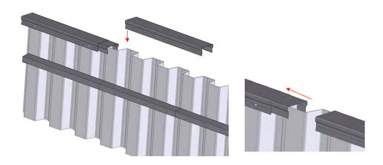
Slide your next cap insert into this cap section, half-in, half-out. This will level the cap section and leave you in a position similar to that in Step 2.
