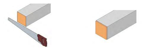
Now cut your joint, and the plastic will be flush with the newly cut wooden face. You can plan ahead and precut all your TimberGuard or cut each joint as you go.
