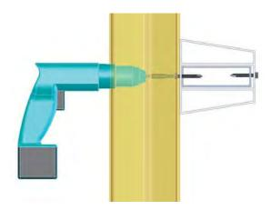
Evenly space the remaining 9 screws over the length of the wale section that does not house any insert (3 shown here). These screws will not be load bearing. They primarily act as a placeholder for your wale until the anchor system is connected.
