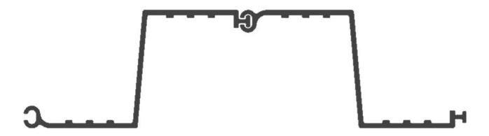
Place your first sheet or pair of sheets on your driving guide and make sure they are in the proper location and orientation for driving. Again, sheet piling installation varies from person to person. The starting location is up to you. It is important, however, to drive your first section plumb, because it will act as a vertical guide for the following sheets.
