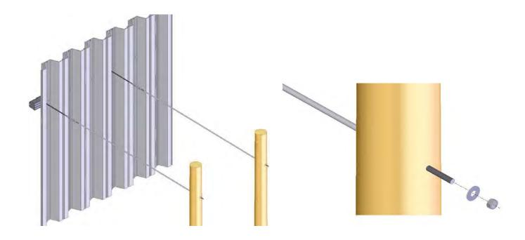
After all of your tie rod components are assembled, use the turnbuckle and a wrench to tighten to the desired tension.
