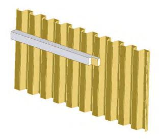
After aligning and leveling your first section, secure your TimberGuard wale to the sheet piling from the back with evenlyspaced lag screws. You do not want to penetrate your joint with screws because you will be securing it with bolts in a later step.
