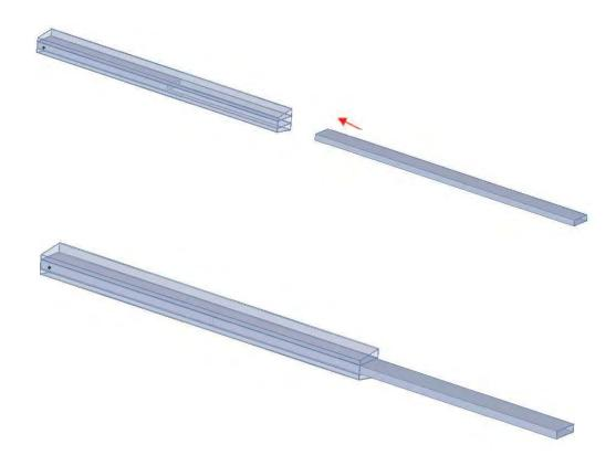
As in Step 2, place this assembly on your sheet piling in the desired position for attachment, and ensure that it is level. You will want to start at one end of your wall and work to the other end.
