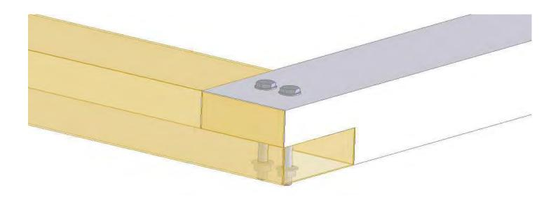
Another aesthetically-pleasing option is a mitered corner. For this example, we will show the steps to create a mitered corner for a 90 degree turn, although you can use this method to create any angled turn by adjusting your cut angle. When you reach a corner, you will want to stop so that your last wale section fits within the straight section of the wall. Make
