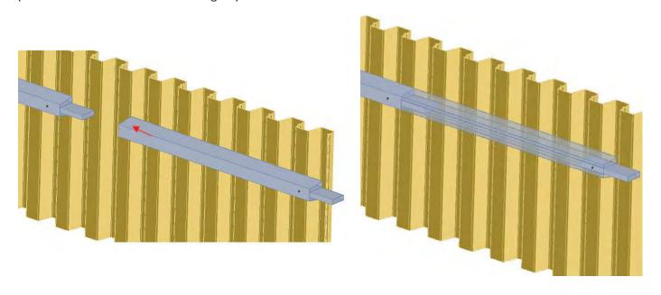
As in the previous step, secure your newly-positioned wale assembly to the sheet piling from the back with the remaining 19 | CMI
