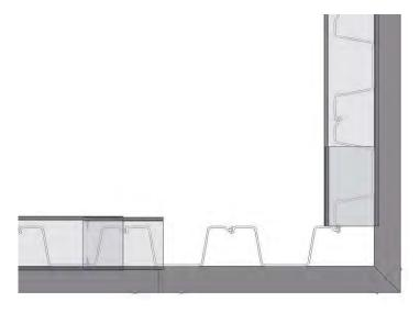
Measure the distance from the farthest point on the cap that you just positioned (this will be the upper flat section) to the last cap section on the flat of your wall.
