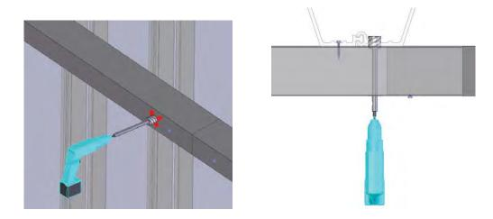
Insert your ShoreGuard coated rod through whatever washer assembly you will be using and into the holes that you have drilled. Shown is a ¾" diameter ShoreGuard Rod, tied back through the wale, with one ShoreGuard beveled washer and one ShoreGuard plate washer.
