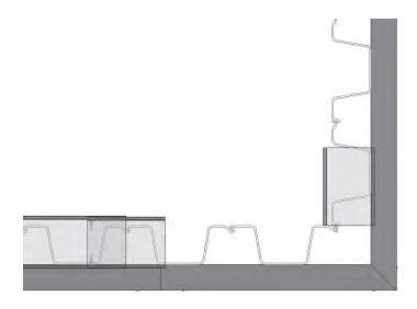
Slide a cap section onto the insert and up to the corner as well. Position these just as you would for final installation. This ensures, in this particular situation, that the cap and wall tightly sandwich the insert on the front side and are hanging over the back just as before.
