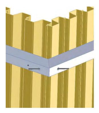
Attach included washers and nuts, oriented as shown. Tighten the nuts.
