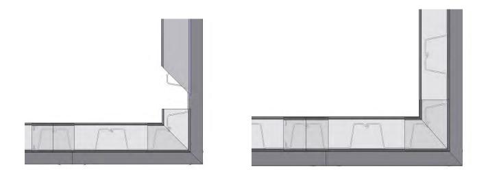
Slide in an 16" insert half-in, half-out of the last cap section. If you will be continuing your wall, this will be used to connect your next cap section. If your wall stops here, then this insert will aid in leveling your cap.
