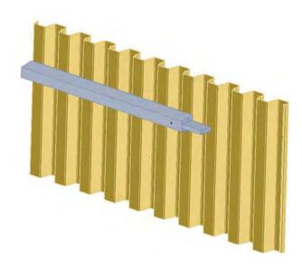
Secure your wale assembly to the sheet piling from the back with the remaining self-tapping screws.
