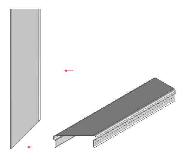
You might want to go ahead and cut your other miter corner piece as well, while you are already cutting. You should make your second corner piece from a new 20' section so that the next splice occurs as far from the corner as possible. For this cut, you will make the matching miter cut 22.5 or 45 degrees from perpendicular, respectively, for a 45 or 90 degree turn. This cut can be made from the end so that no measurement is necessary.
