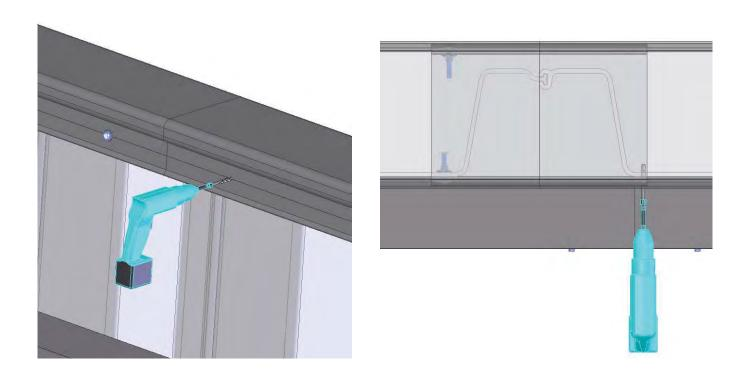
Repeat this process for the rear of the wall. Again, in this case, you want to make sure that you do not drill through the wall, only the cap and insert, so that they can be securely fastened, and the cap will remain in direct contact with the front wall face.
