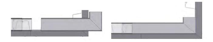
After your cap section and corner insert are in place, slide your matching miter cut cap section (the one from a new 20' section) onto the exposed insert.
