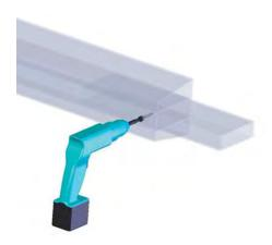
Slide your newly-created wale assembly over the exposed insert section of the previously-hung wale assembly. You will use each hung wale assembly as a guide for the following wale assembly. You will still want to ensure that each is correctly positioned and level before attaching to your wall.
