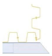
Insert the appropriate corner insert, in this case a 90 degree corner insert, into the wale section.
