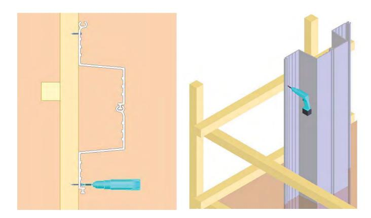
Continue this process for the first straight run of your wall. There should be enough play in the locks and flexibility in the sheets to ensure that each sheet can install in the proper position.
