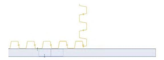
Extend a line from the angled face and transfer a construction line to the wale section using a marking device.
