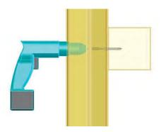
These screws will not be load bearing. They primarily act as a placeholder for your wale until the anchor system is connected.
