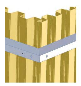
Insert the 16" threaded rod through both holes.
