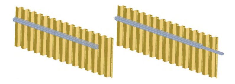
At this point you will secure your unattached wale and insert to the sheet piling. From the back, fasten your unattached wale and insert by evenly spacing all 10 of your self-tapping screws. While you can penetrate the inserts, do not attach the exposed section of the insert, so the next wale piece can slide over the insert.
