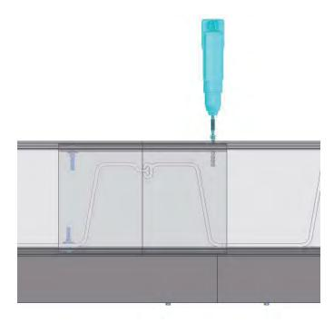
Hand-tighten the front side first to ensure good solid contact, followed by hand tightening the rear side, and then fully tighten both. Remember, in this scenario, we have chosen to sandwich the front face of the wall in as well.
