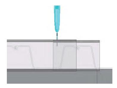
After both holes have been drilled, secure them with the cap bolts and washers, in the order shown. The PVC washers ar
