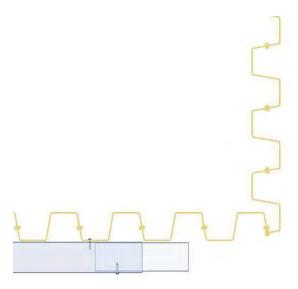
You will want to slide the next wale section on, in order to identify and mark where your miter cut needs to be made.
