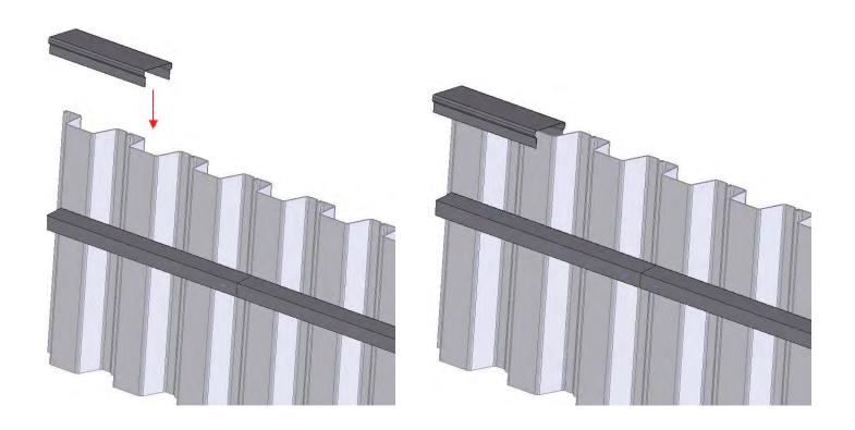
Place a 20' insert onto the wall so that it touches your already positioned 10' insert.
