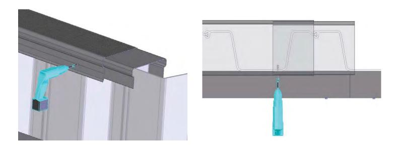
Repeat this process for the rear of the wall. In this case, however, you want to make sure that you do not drill through the wall, only the cap and insert so that they can be securely fastened, and the cap will remain flush with the front wall face.
