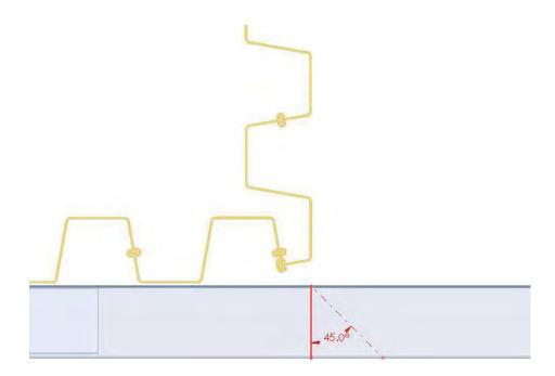
Slide off your marked wale section and cut your angle. You might want to go ahead and cut your other miter corner piece as well, since you are already cutting. You should make your second corner piece from a new 20' section so that the next splice occurs as far from the corner as possible. For this cut you will make the matching miter cut 22.5 or 45 degrees from perpendicular, respectively, for a 45 or 90 degree turn.
