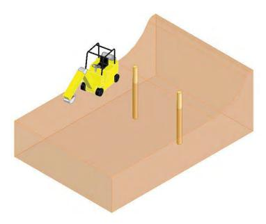
In cases where excavation is undesirable, there are other types of anchors that can be driven or screwed into the ground, leaving the exposed topside virtually undisturbed. The type pictured below has a mechanism that extends when sufficient pressure is applied to the rod, securely holding itself in place. These types of anchors can also have load checking devices, to ensure that they are installed with a firm footing.
