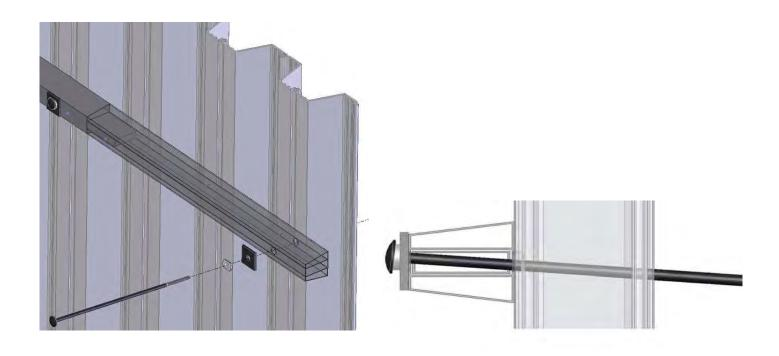
Screw the appropriately threaded end of the included turnbuckle onto the threads of the coated ShoreGuard rod. The coated rod section is reverse-threaded to allow your tie rod system to be tightened with the turnbuckle after assembly.
