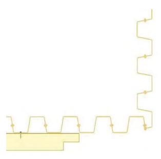
If you haven't already done so, you will want to take your measurements for cutting your first corner wale piece. An easy way to do this is to use a section on which the joint cut has already been made. Place it on the wall as if you were going to connect it to the previously hung wale section. Extend the line from the angled face, and transfer a construction line to the wale section using a marking device.
