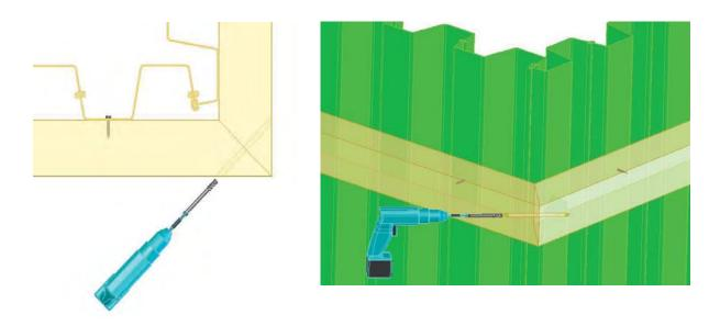
Make a countersunk hole concentric with the hole that you just drilled, and deep enough to house the nuts and washers. It should be wide enough to accommodate the washers you have chosen.
