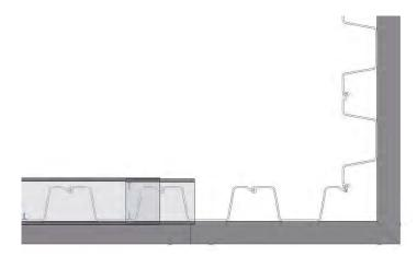
Identifying the proper location for your miter cut is very important for a quick, simple, and attractive wall. There are many ways to accomplish this, but one of the simpler ways is as follows: Place a cap insert onto the turned wall section and slide it as far into the corner as possible.
