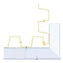
Slide your second cut wale section onto the exposed corner insert.
