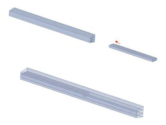
Secure this piece through the front with a self-tapping screw. This is just to keep the insert from moving inside the wale section.
