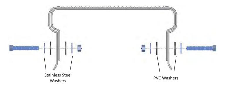
Hand-tighten the front side first to ensure good solid contact, followed by hand tightening the rear side, and then fully tightening both. In this scenario, we have chosen to sandwich the front face of the wall in as well.
