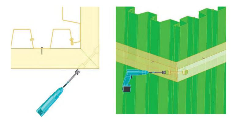
Insert the threaded rod into the drilled hole. It is a good idea to make sure the ends of the rod do not extend outside your wale. You may want to consider cutting them off if they do. Removing this extrusion will help protect the rod from the elements, as well as improve the aesthetics of your wale.
