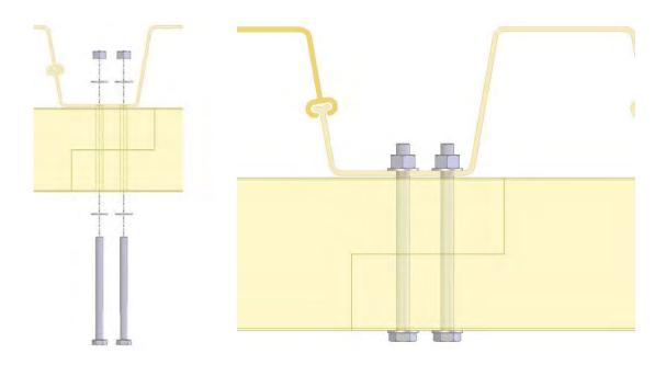
The process is the same if your joint lands on a gap. However, you will only bolt through the TimberGuard, not the sheet piling.
