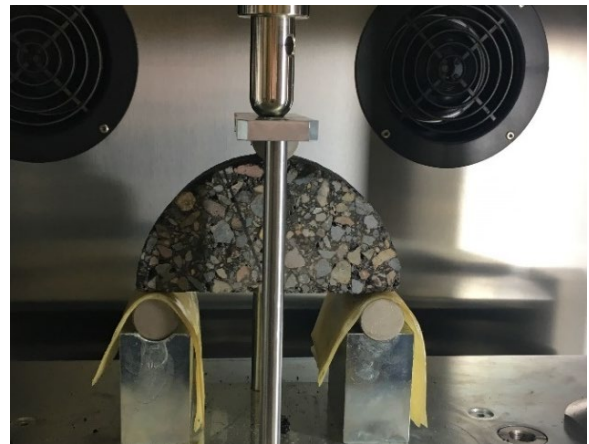
Figure 20 – SCB Test Set-up
