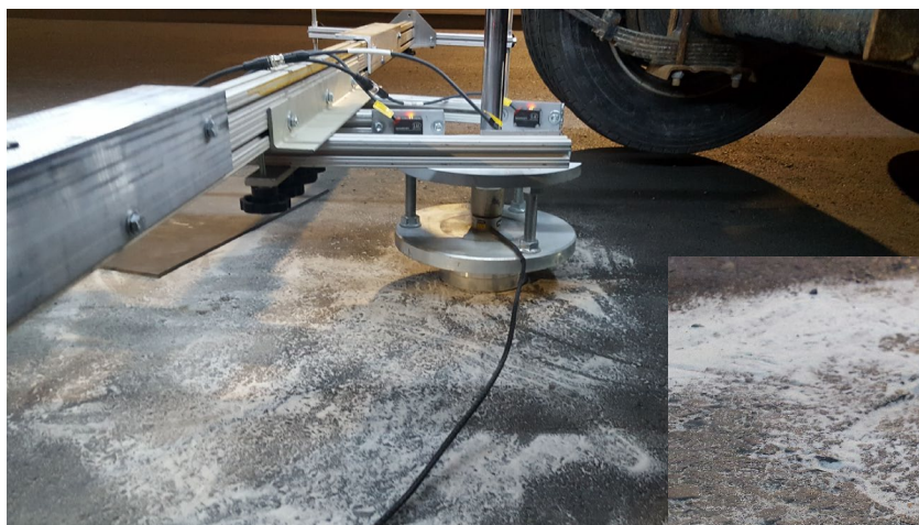
Figure 14 6 in. diameter flat plate - Repeated Load and Static Load Creep Test
